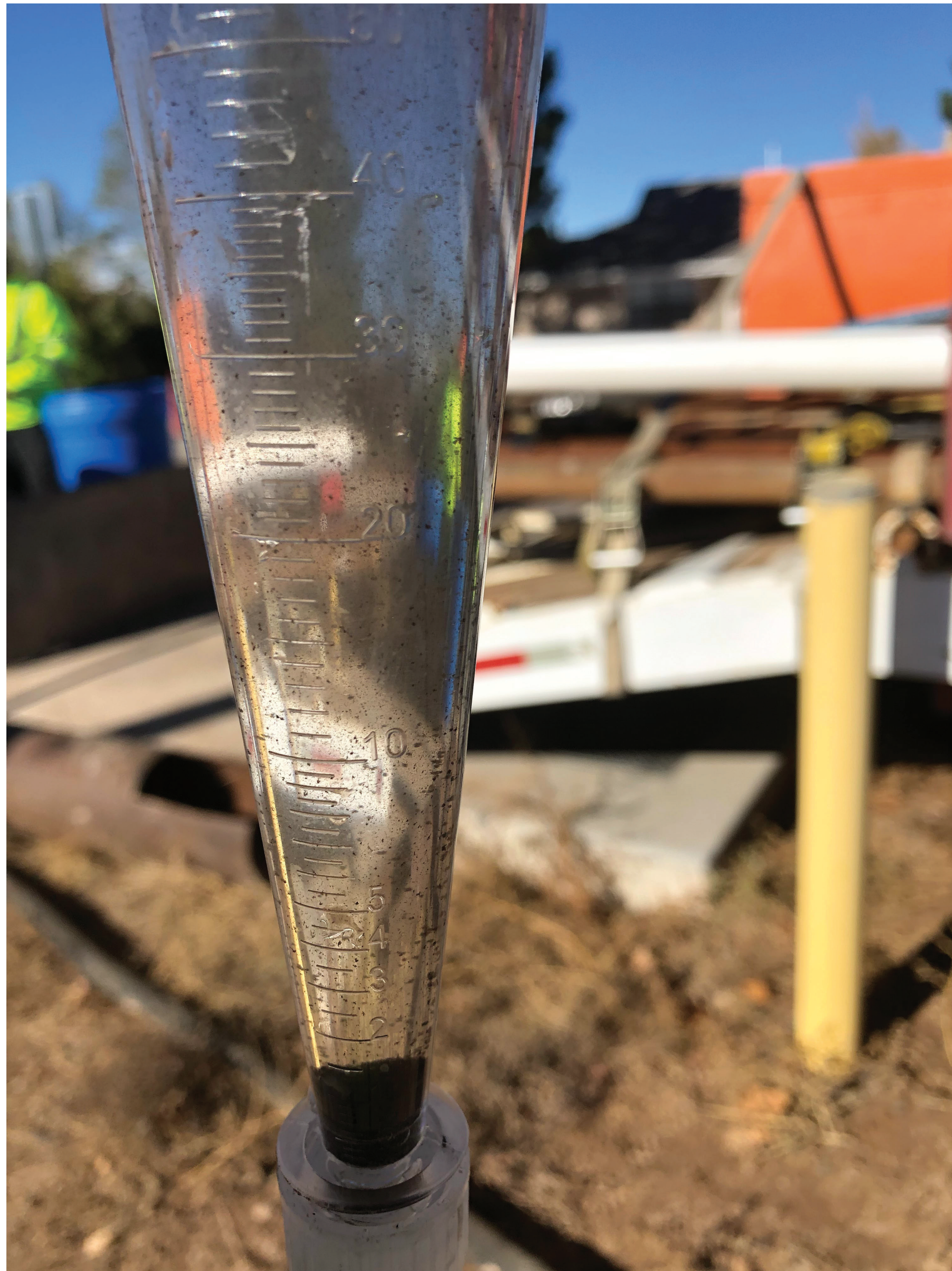
Extraction well KAFB-106239 final turbidity
